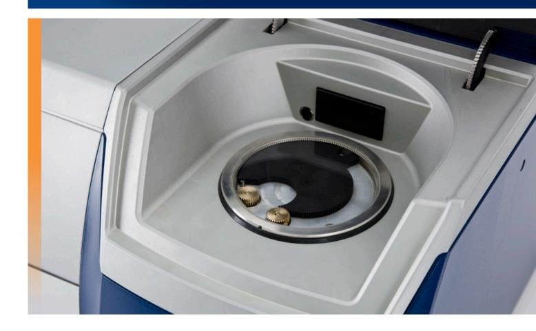
The NIRS™ DS 2500 analyser helps millers to boost yield by giving unique levels of accuracy regarding ash as well as highly accurate measurements of protein, moisture and colour.
